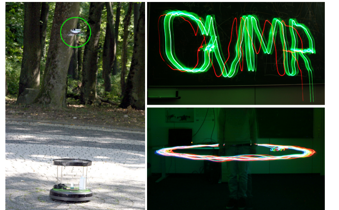
(b) MAV tracked and controlled by a mobile ground robot. (c) Light paintings of the flights evaluated in Section IV.
